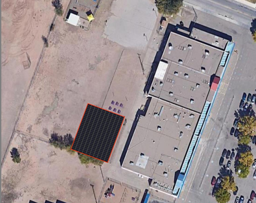
Main Building Playground Array 175 kW DC Est 85% Offset
